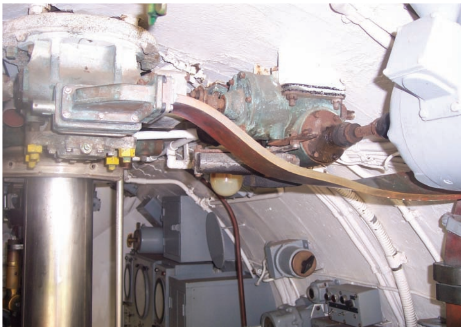
Figure 3: A rectangular waveguide in the conning tower of a WWII U.S. Navy Submarine. (Source: Author's private collection)
